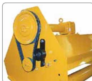
Tendicinghie registrabile. Adjustable belt tensioners.
