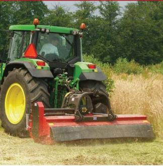
**Professional flail mower for heavy vegetation** The Landmaster is specially designed to mow green manure crops and stubbles, which makes it also suitable for maintaining rough terrain.
