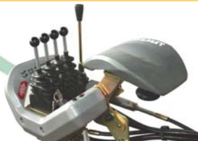
Multi-lever Low Pressure hydraulic assisted controls
