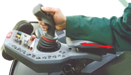
Single-lever Low Pressure mixed (elec. + hydr.) controls
