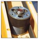
Big pulley diameter (130 mm) and KEVLAR belts (57 mm high) to get a better power transmission.
