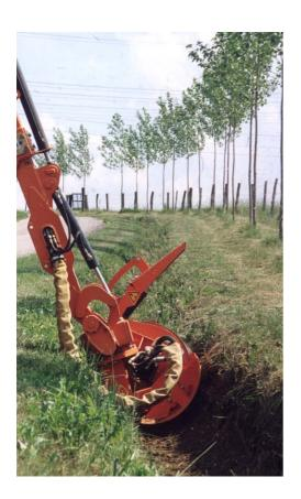
The ditch-cleaner helps ditches play their role : make it easier for the water to flow, in order to keep the road as dry and safe as possible.
