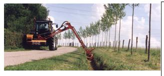
Ditch-cleaner can be easily fitted to Noremat machines Tonica, Optima, Magistra and Maxibra, through the quick-coupling system.
