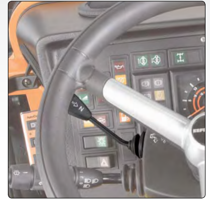
Directions can be changed fast yet smoothly using the F/R shuttle .
