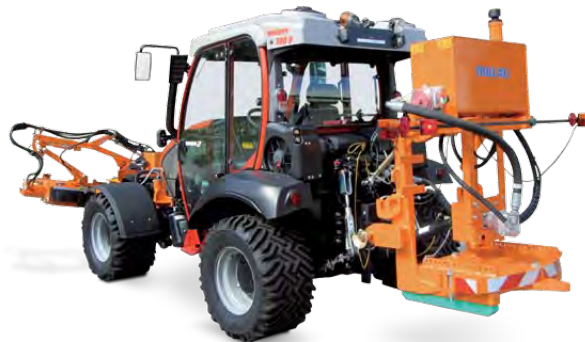
1 Extension arm boom flail mower 2 Hydr. drive unit
