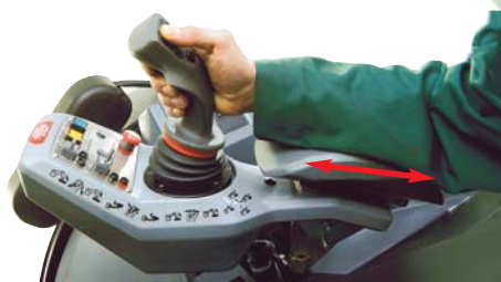
Single-lever Low Pressure mixed (elec. + hydr.) controls
