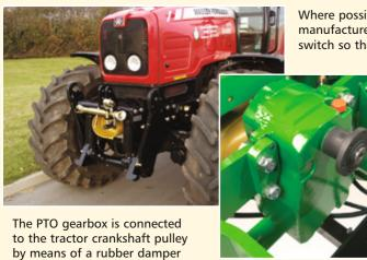
preventing vibration. Similarly the "soft start system" uses an electro hydraulic multi-plate clutch inside the gearbox to provide smooth power engagement to the front PTO. Oil pressure for the clutch is supplied by an intergrated pump in the gearbox which is driven by the input shaft.
