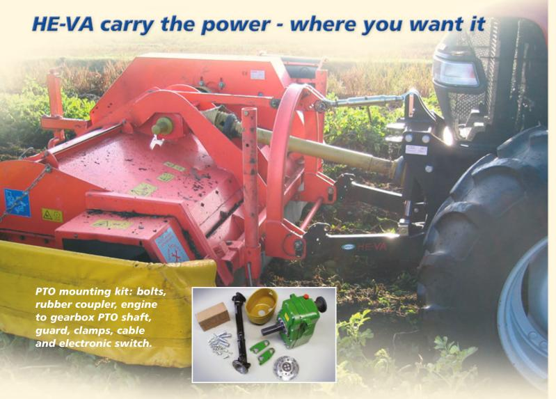
HE-VA PTO's can be fitted to most linkages.
