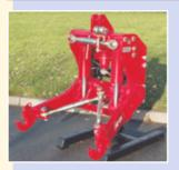
The 4 or 5.5 ton Multi-fit linkage incorporates all the standard features of 2.5 to 5.5 ton linkages but is manufactured without full length side plates. This multi-purpose linkage has short side plates with multiple attachment holes so that it can be adapted to fit various machines and tractors where a three point linkage is required, e.g. trailers, slurry tankers & 4 wheel drive vehicles
