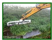
Michaelis cutter buckets are designed for mounting on backhoes and excavators and come in varying cutting widths from 2.2m to 5.0m. This means that the Michaelis cutter bucket can be ordered to suit the size of the machine it is to be mounted on and the work that is to be carried out.
