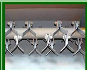
The flail mower with a working width of 100 cm is equipped with a hefty rotor shaft with 6 mm Y blades and a robust, spacious flail hood. This facilitates a high throughput and fine chopping. The height adjustment, which ranges from 45 to 100 cm, is operated via the front wheels.
