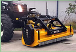
The popular choice for roadsides and orchard prunings is the ORSI WGR series. Available in cut widths from 1.5m to 3.2m the popular choice has been the 2m SX series. This WGR is designed strong for the rigors of road shoulder maintenance and has 4/5 drive belts positioned out of harms way.
