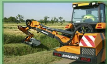
Floating mowing head position from Noremat. This system is switched on and off from the operators seat and even when activated the operator retains control over the cutting head position.
