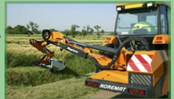
Floating mowing head position from Noremat. This system is switched on and off from the operators seat and even when activated the operator retains control over the cutting head position.
