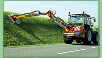
Reverse break-back acts in the event of an erroneous manoeuvre, the arm gives slightly forwards, thus protecting the cylinder from breakage. This system also comes into action if the driver is forced to break heavily when working on a steep downhill slope.
